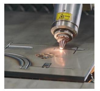
1. The new, highly dynamic laser bevel cutting unit Bevel-U makes possible the preparation of precise and consistent bevel parts – a great advantage for edge preparation for automated robot welding
