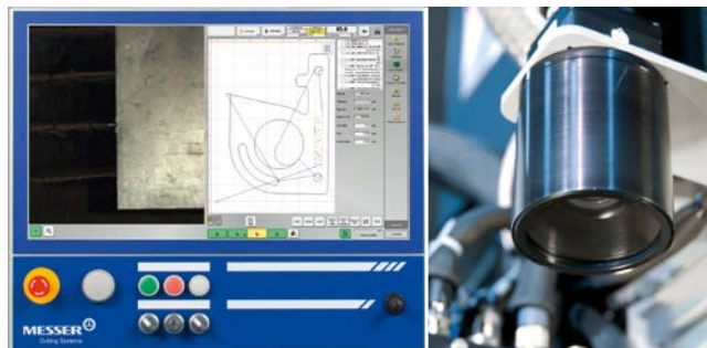
Video camera (right) allows for fast, accurate plate alignment
