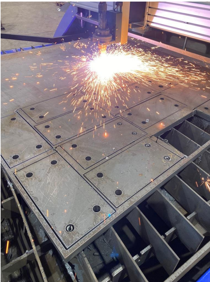
Photo 3: The machine is equipped with the new power source Q 1500 plus from Kjellberg. Thanks to the Q-Hole technology, precise holes can be cut with a ratio of 0.75:1.
