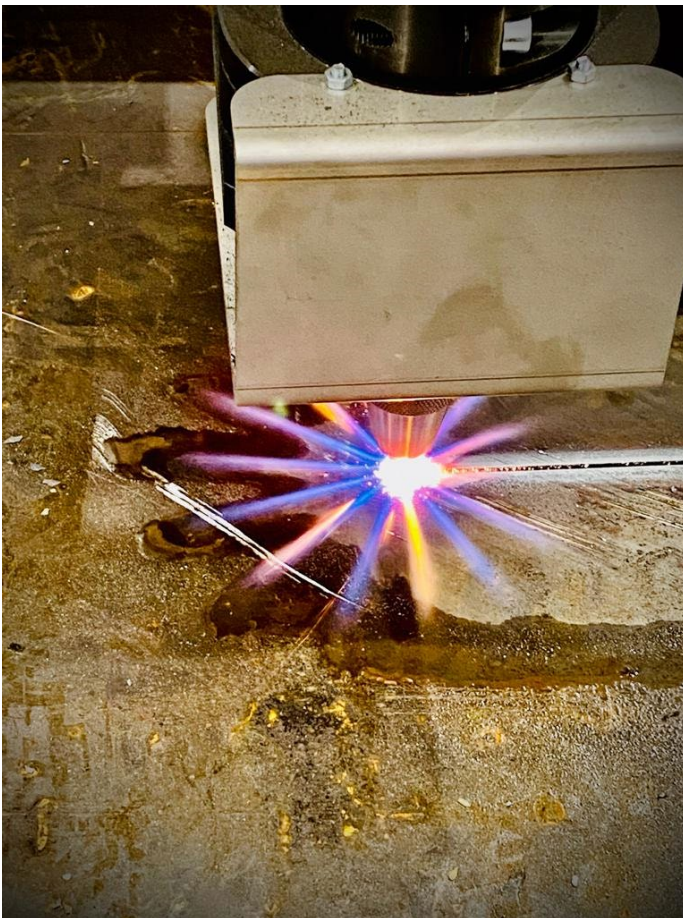
Photo 2: With the ALFA oxyfuel torch, sheet metal thicknesses of up to 100 millimeters can be processed.
