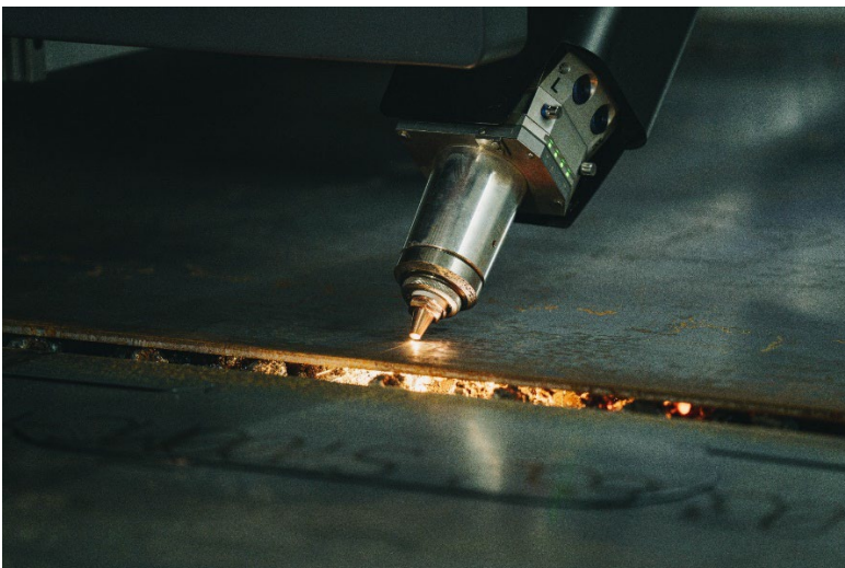
Image 9: The new, highly dynamic laser bevel unit Bevel-U enables the production of precise and repeatable bevel parts - a major advantage when preparing edges for automated robotic welding. © Messer Cutting Systems
