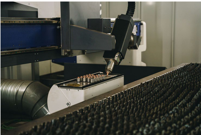
Image 2: A feature for the automation of the ELEMENT 400 L is the Laser Nozzle Control (LNC). It automates the set-up work quickly and reliably, thus ensuring maximum quality and productivity. © Messer Cutting Systems
