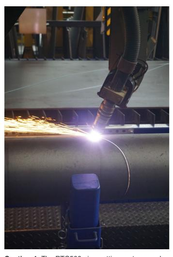
**Caption 4:** The PTC500 pipe cutting system can be used to process round pipes with a diameter of up to 500 mm. The Skew Rotator Delta ensures precise bevel cuts for weld seam preparation. © Thöni Industriebetriebe GmbH
