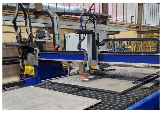
Caption 5: The ALFA oxy-fuel torch cuts effectively right to the edge of the plate, ensuring better material utilisation. © Thöni Industriebetriebe GmbH
