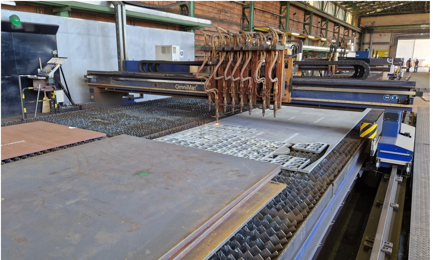
Image 5: The OmniMat with 8 oxyfuel torches.
