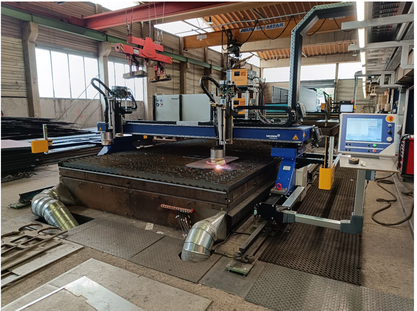
Image 3: The new MultiTherm with 2x HiFocus 280ineo.
