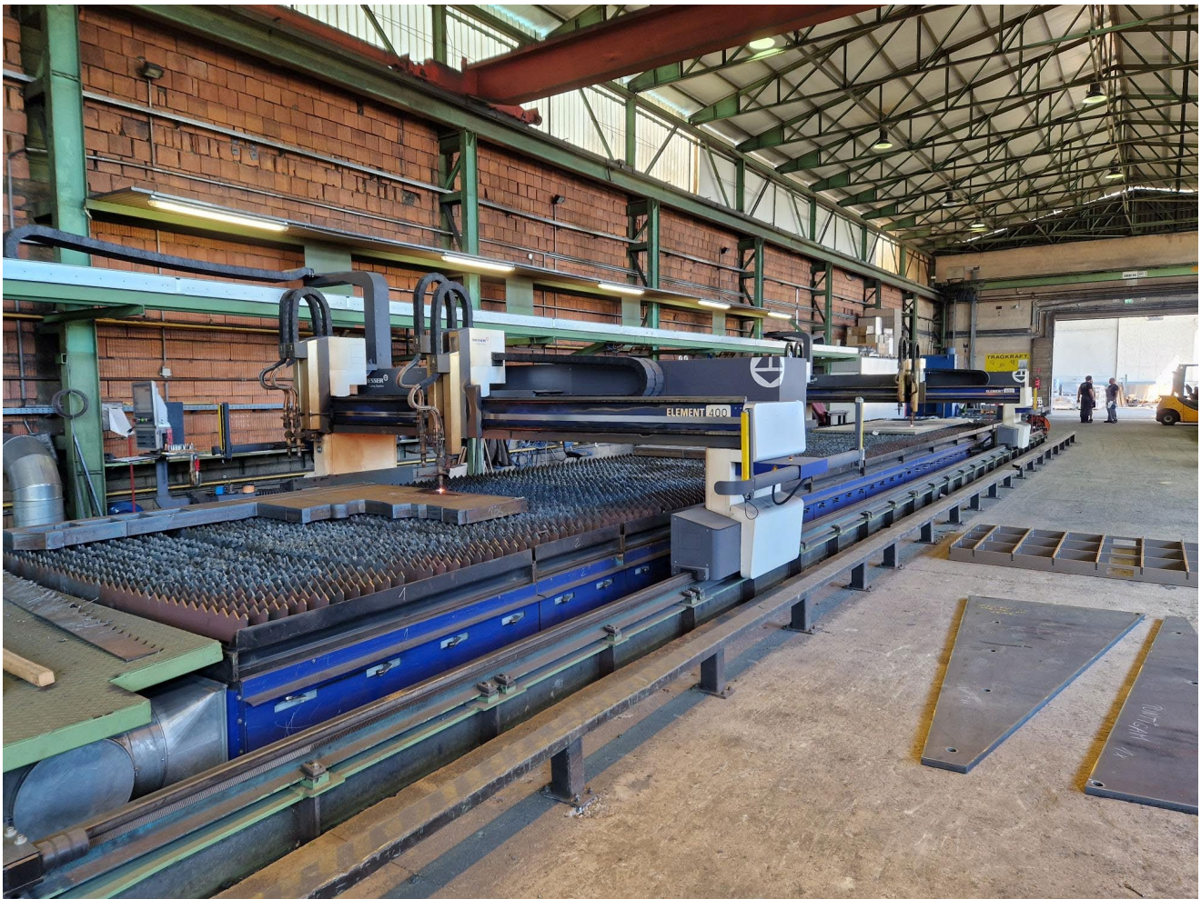
Image 4: Two ELEMENT machines, each with 4 ALFA oxyfuel torches on a track.
