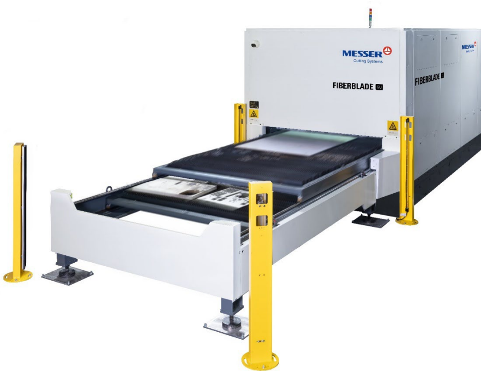
Image 4: The parallel change-over table ensures a smooth material change and thus significantly shortens the production time.
