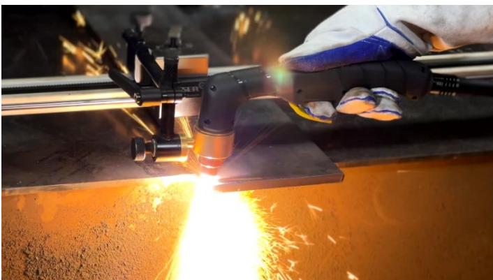
Photo 3: The Plasma Cutter – here in combination with the mechanical cutting guide StableCut – ensures high productivity in plate processing.
