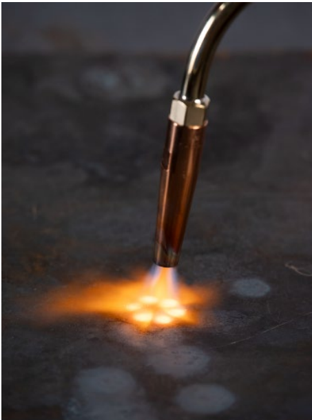
Photo 1: To take the special characteristics of Hydrogen into consideration, special torches and nozzles have been developed. In action: surface heating torch with new heating insert F-H.
